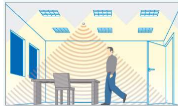
Presence detected, insufficient daylight, all lights on.
