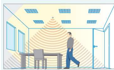
Presence detected, sufficient daylight, lights off.
