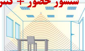
No presence detected, daylight, lights off.
