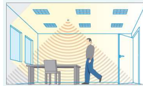
Presence detected, sufficient daylight, lights off.
