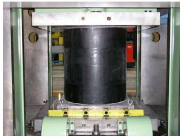
Load test of HDC foundation element in protection sleeve
