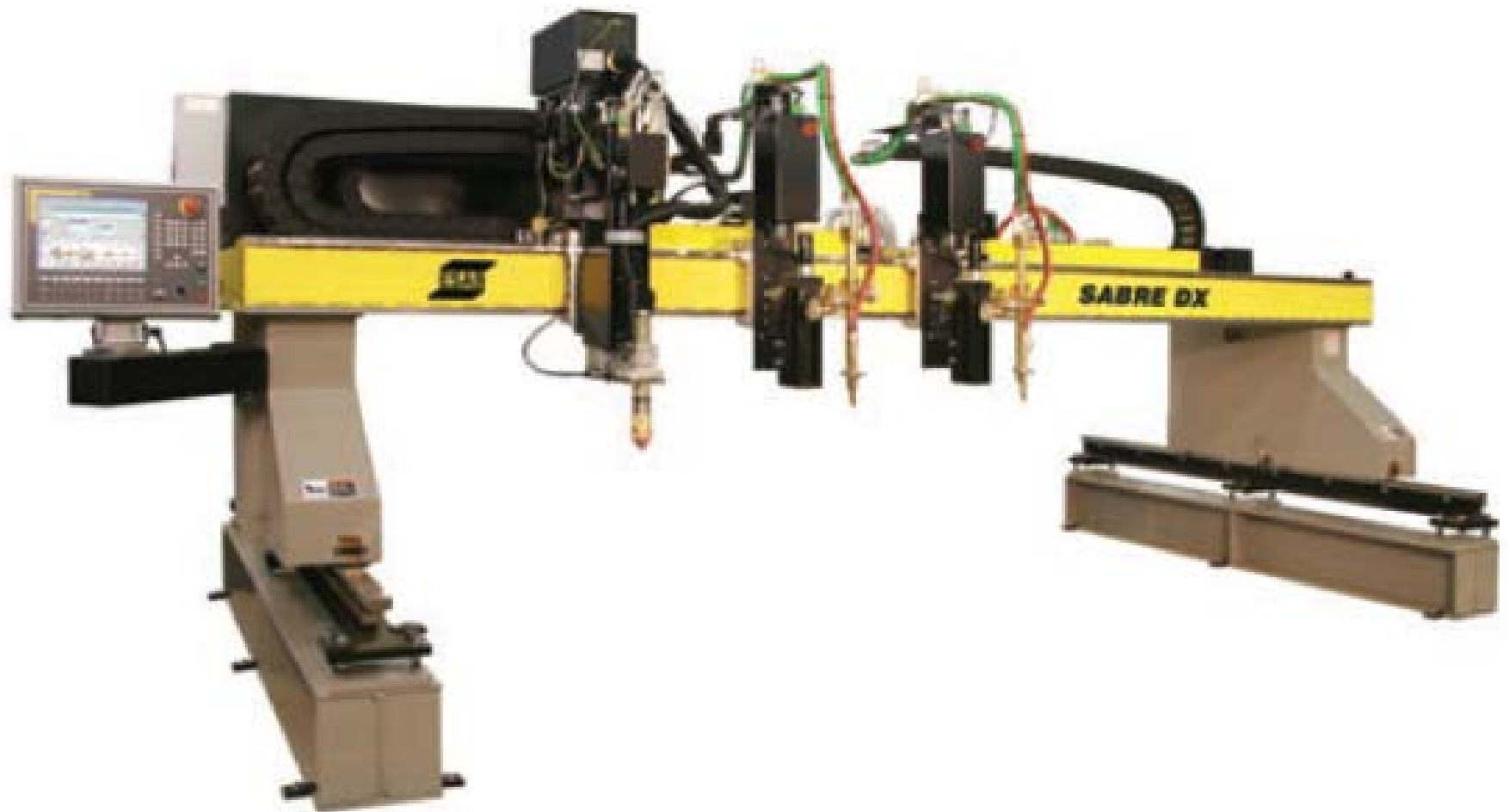
FIGURE 7-7 Multiple head cutting machine. ESAB Welding & Cutting Products
