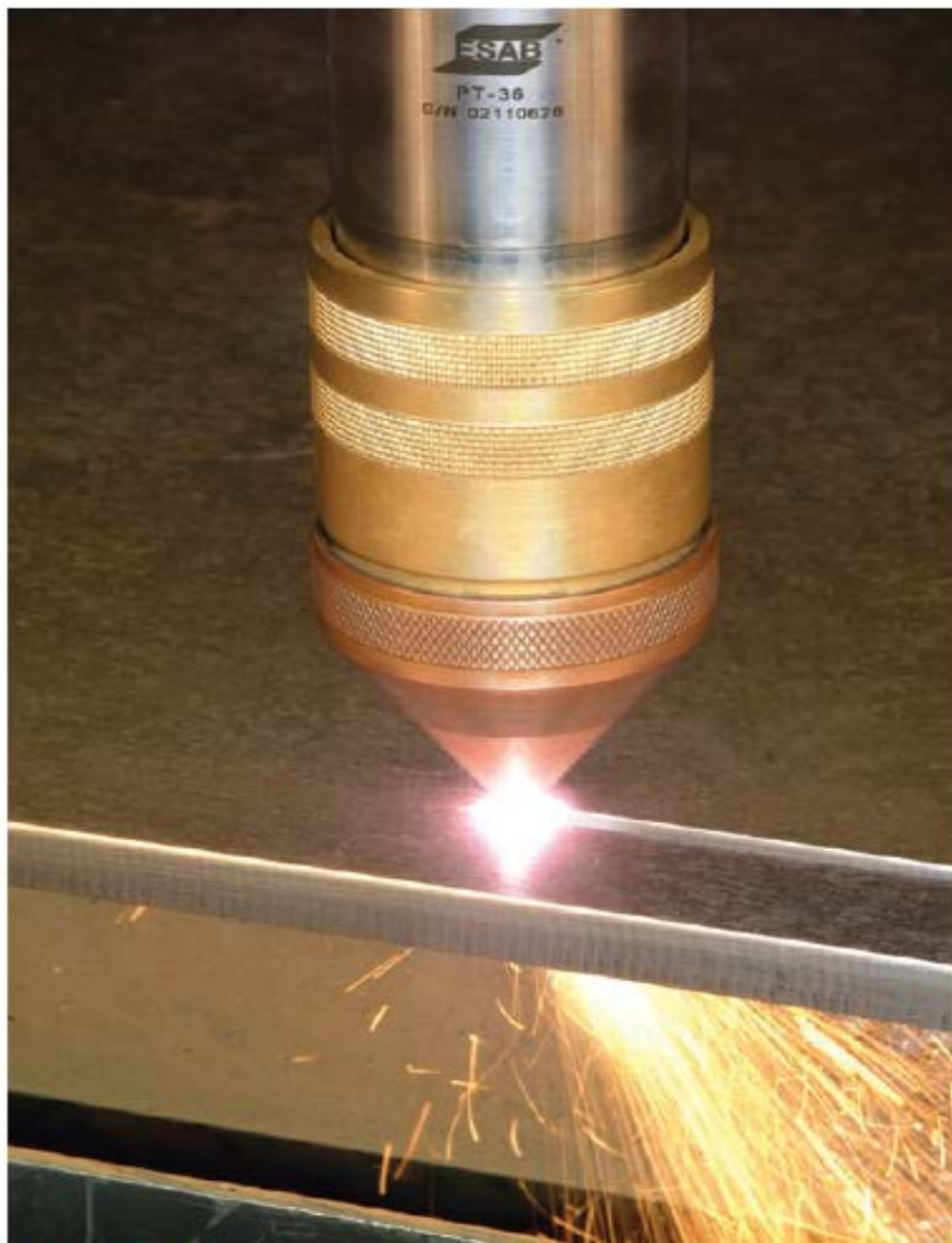
FIGURE 8-23 When the standoff distance is correct, as with this machine cut, almost no sparks bounce back on the cutting tip. ESAB Welding & Cutting Products
